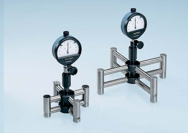
Cross sleeve with runners for dia. 130-500 mm for deep bores or through bores, alignment in the bore is made through the 4 runners
