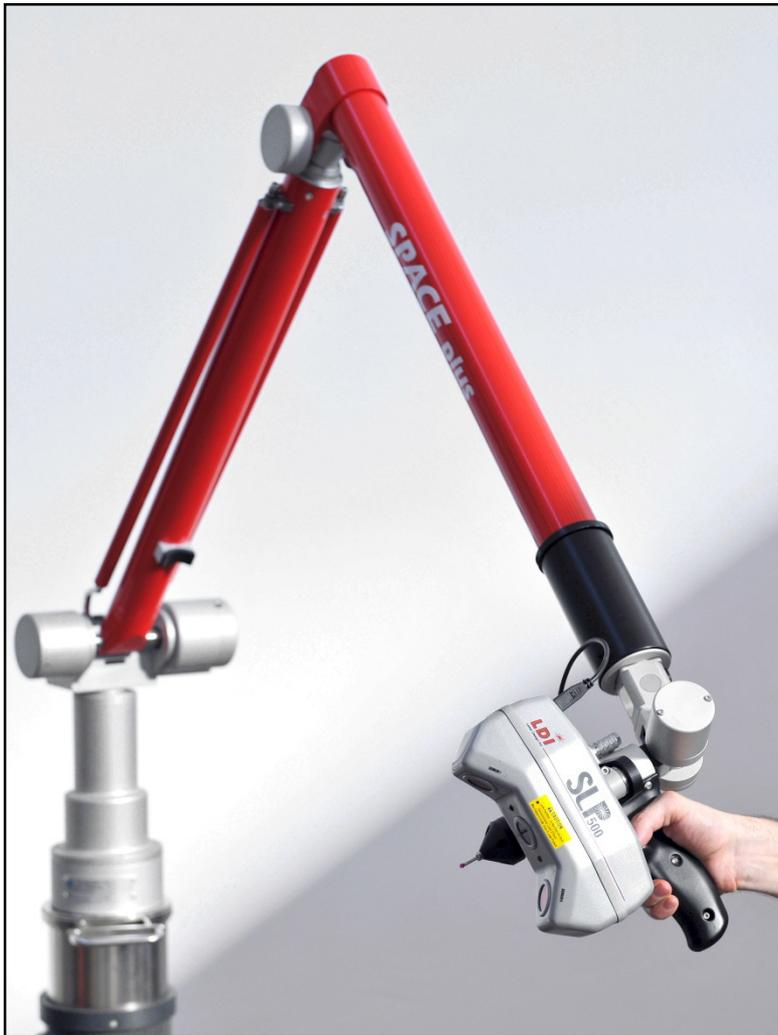
**SPACE SCAN** system is the combination of the **SPACE 7 AXES ARM + HI-END Scanner, SLP by LDI**, a new family of line-range laser probes that are ideal for complex-profile contour scanning.
