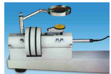
Calibration of lever type dial
