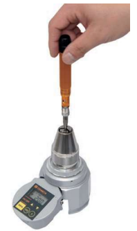
Torque checking figure for BMRD torque screwdriver for small screws with BTGE-G
