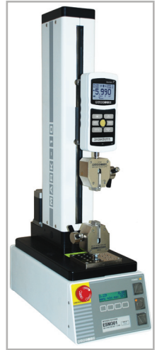
Shown with an ESM301 test stand and G1061 wedge grips
