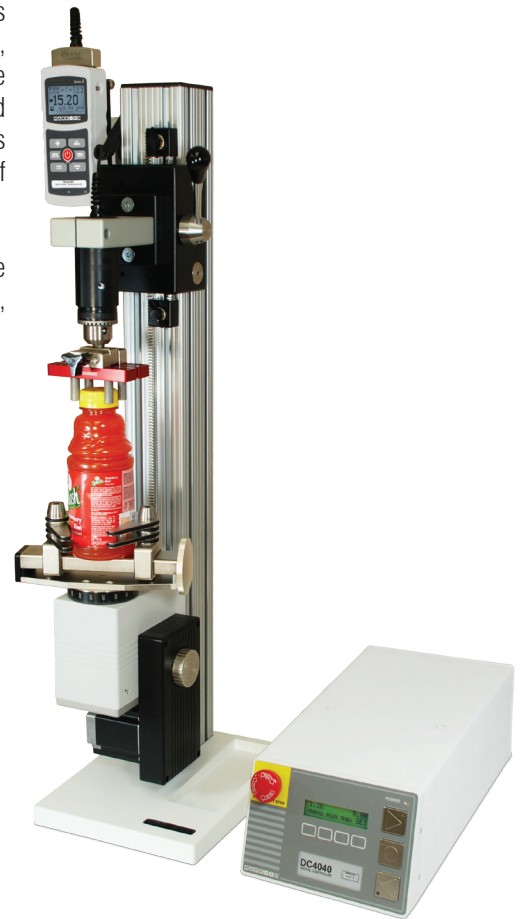
^ The TSTM-DC is shown in a cap torque test, with a Series R50 torque sensor, M5i force/torque indicator, G1023 universal closure grip, and G1053 cap grip
