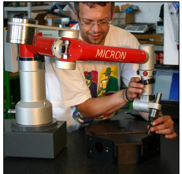
**MICRON** arms, will be suitable for 3D quality inspection of any parts, whether on a simple granite or steel table, or directly in the machine tool, thanks to the portable tripod that can be positioned easily close to the machine.
