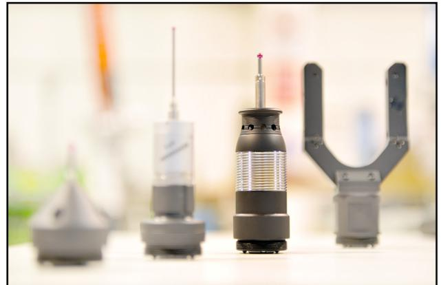
All the available probes fits the same mechanical mount of the standard **MICRON** version and are interchangeable. The precision mount is extremely repeatable and allow to switch from one probe to another without recalibration.
