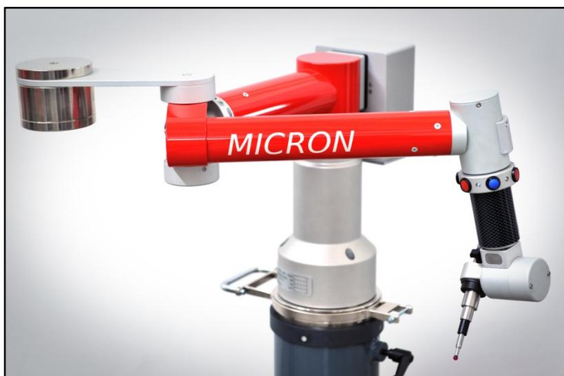
The **MICRON** arms are designed to be fixed on a tripod with wheels that is adjustable in height and has a shelf that enables measurement of the part within, for example, the machine tool. They can be also fixed on other support equipment including granite table.
